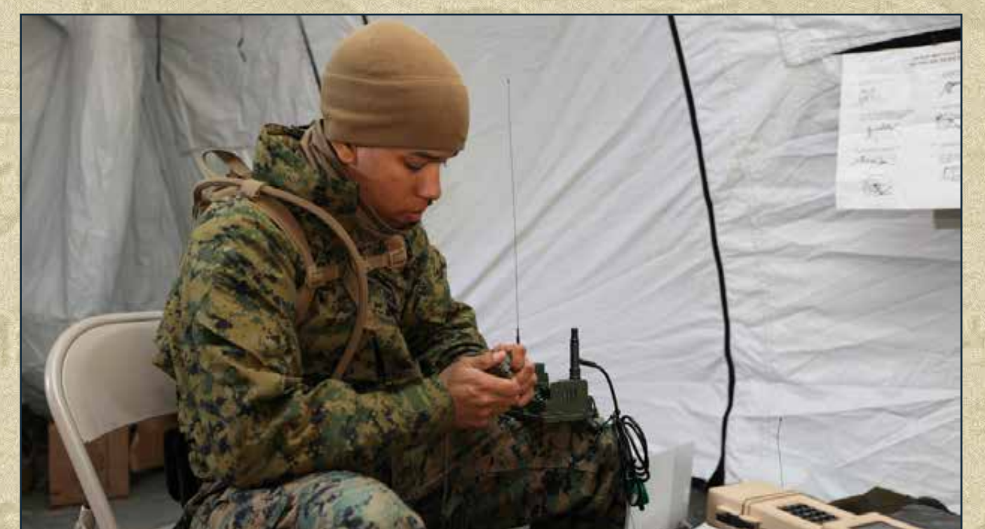
PFC Ariel A. Tolentino, a radio operator with the 22nd Marine Expeditionary Unit ground sensor platoon prepares "unattended static" ground sensors used to detect movement, sounds, and vibrations in the field. (U.S. Marine Corps)
