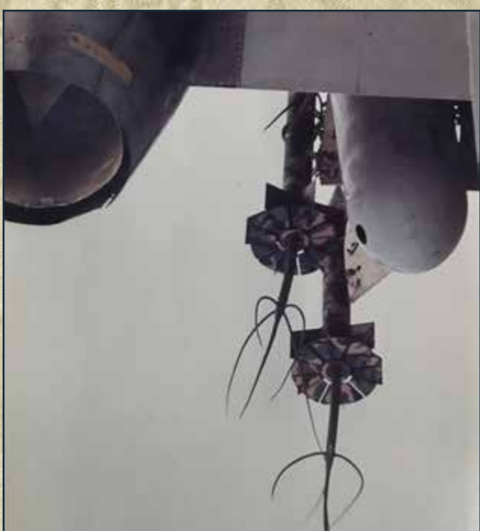
Two Air Delivered Seismic Intrusion Detectors on the pylon of a Navy OP-2E aircraft prior to their being deployed in Laotian airspace over the Ho Chi Minh Trail. (National Archives)
