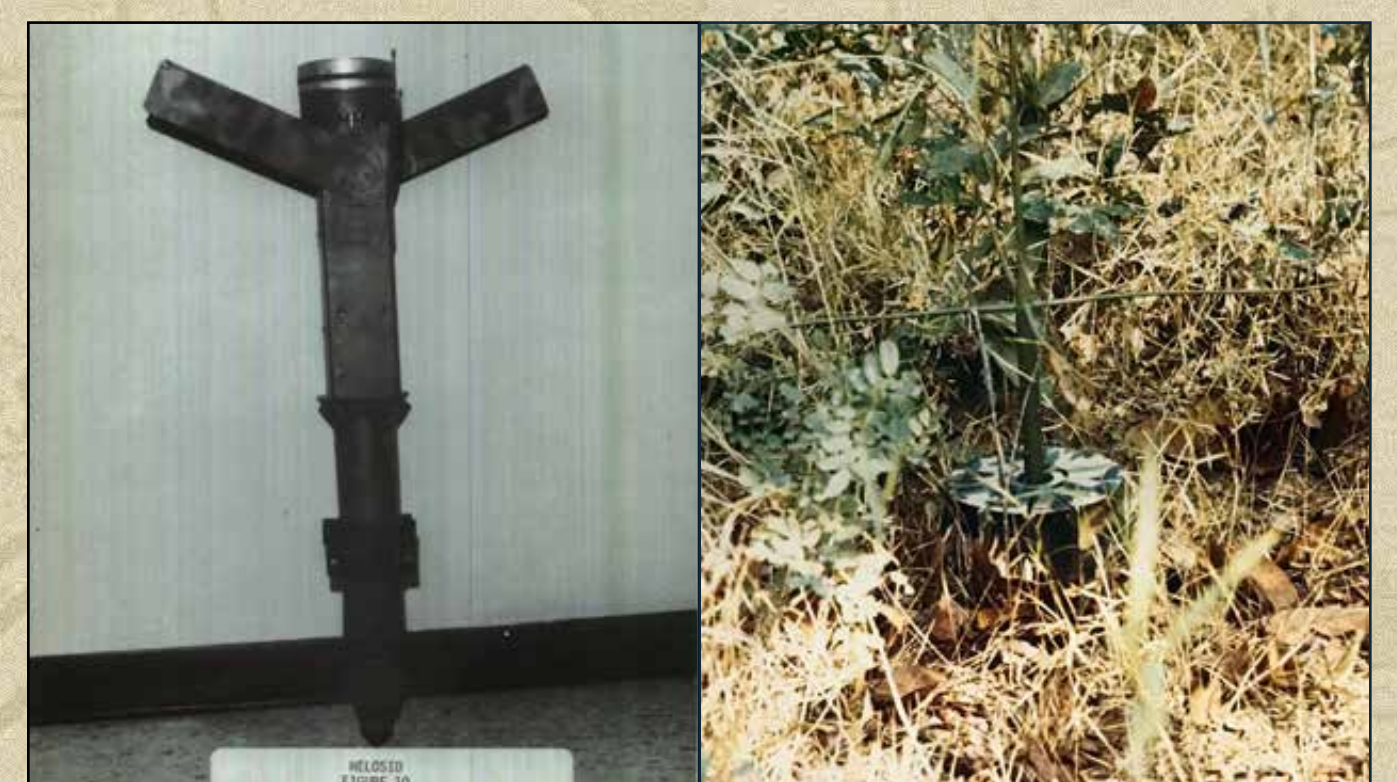
Left: The Helicopter Emplaced Seismic Intrusion Detector. A seismic sensor detects vibrations and movement from passing footsteps or vehicles. It is designed to be launched from a pod attached to a CH-3 helicopter or tossed from its side door while the aircraft is hovering. (Defense Technical Information Center)
